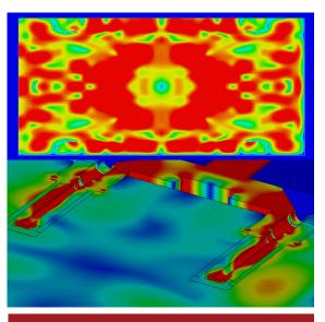
Laboratory ovens Simulation of Power Flow
