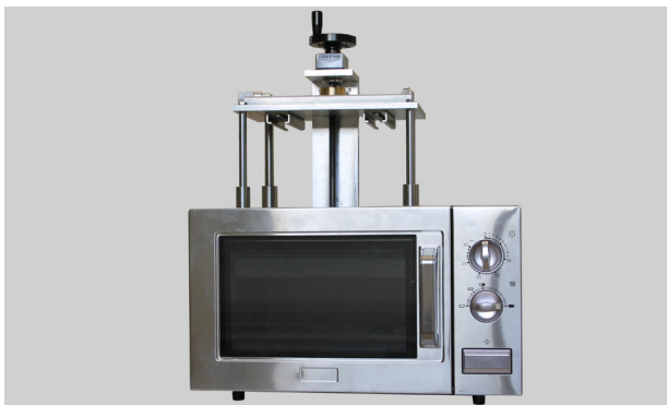
Test device: Microwave Chamber 500 W / 2450 MHz
