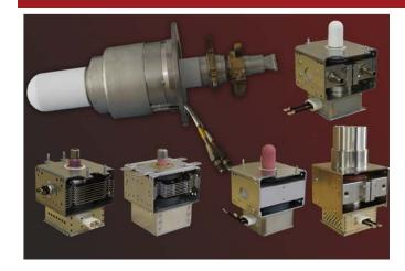
Fricke und Mallah supplies numerous versions of top-class magnetrons for high frequency applications. These play a central role in the generation of electromagnetic energy. We supply them in the frequency ranges 915, 2450 and 5800 MHz. The output power, depending on the design and frequency range, is available from 300 W to 100 kW.
